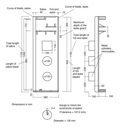
Figure 16. Gauge for checking weapons
