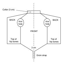
Figure 14. Foil: conductive jacket
