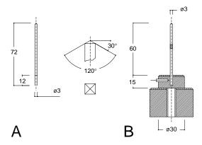
Figure A.2. High speed dynamometer for test of cloth resistance to perforation
