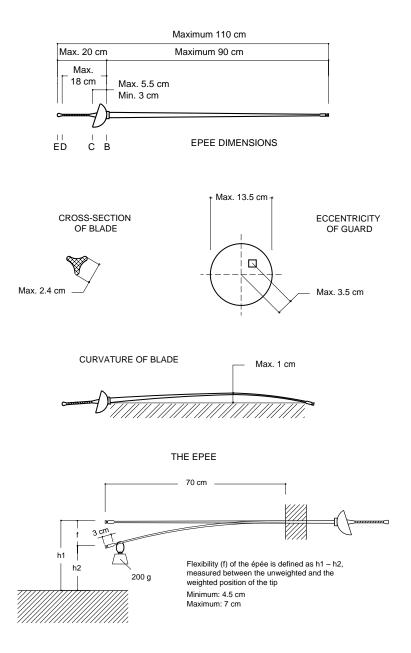
Figure 9. Epée dimensions and flexibility
