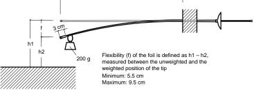
Figure 8. Foil dimensions and flexibility
