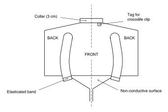
Figure 15. Electric sabre: conductive jacket
