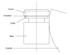
Figure 11. Epée: details of tip of point
