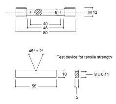
Figure A.6. Test devices for traction and tensile strength
